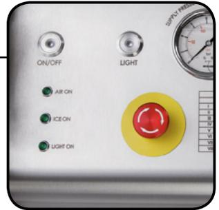
10. Turn the machine ON [press the ON/OFF button].
