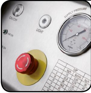
9. Check to make sure that the machine is in the normal operating position [the emergency stop button is pulled out].
