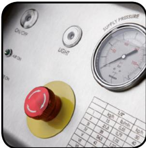
15. **“Light button”** (only when machine is equipped with a light gun) - to improve visibility during blasting turn on the “Light button” on the control panel.
