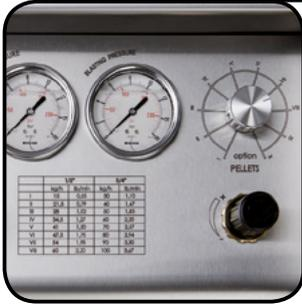
13. Adjust the dry ice consumption [kg/h / lbs/min.] and the blasting pressure [bar/psi] - the value is shown on the pressure gauge.
