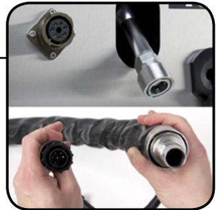
2. Plug the blasting hose couplings into the socket on the front of the machine and the blasting gun, respectively. **Check to make sure the hose couplings are correctly connected.**
