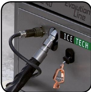
3. Connect the signal cable at both ends of the blasting hose with the sockets on the front of the machine and the blasting gun.
