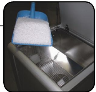
**Please note:** It is recommended that **you run the hopper empty** before each filling to enable the operator to see whether “snow” or lumps appear in the dry ice. These can prevent a continuous supply of dry ice to the dosing unit.
