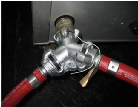
The first option is a 3-way Universal Claw Coupling. This allows the use of two  $\frac{3}{4}$ " airlines to carry volume to the machine or after cooler dryer and combine the volume at the air inlet. Two  $\frac{1}{2}$ " airlines can also be used to carry volume to a three quarter inch or smaller machine in a plant.
